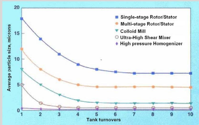
In this particular dispersion, the Ultra-High Shear Mixer outperforms the colloid mill and other rotor/stator designs. The average particle size achieved in the UHSM approaches that of a high pressure homogenizer.
